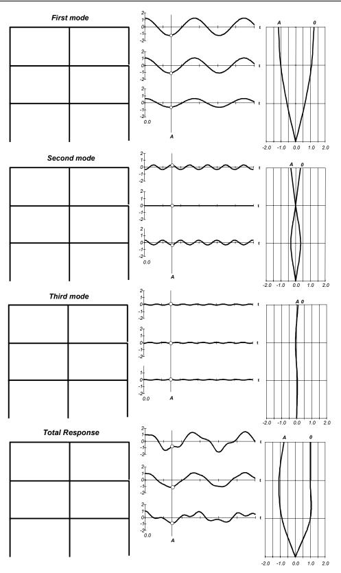
Fig. 2 - Response to initial displacement conditions. Case (a)
