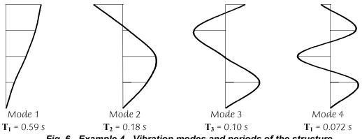
Fig. 6 - Example 4 - Vibration modes and periods of the structure
