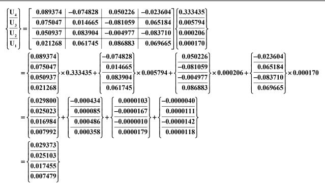
To obtain the forces caused by the explosion at the same instant for all the structure, the structure stiffness matrix is multiplied by the displacements obtained:
