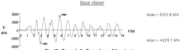
Fig. 13 - Example 5 - Base shear of the structure
