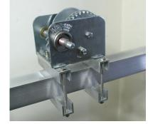
**Step 9:** Attach the cable guide pulley approximately 10" above the winch using one aluminum u-channel and  $1/4 \ge 5-1/2$ " bolts and flange nuts.
