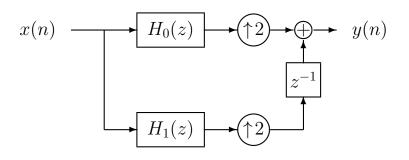
Note that in the last block diagram, the filters operate at the slower rate, and the filter inputs are not zero. Also note that the filters  $h_0(n)$ ,  $h_1(n)$  are each half the length of the original filter h(n). The adding node in the last diagram does not incur any actual additions — it implements an interleaving of the two branches.
