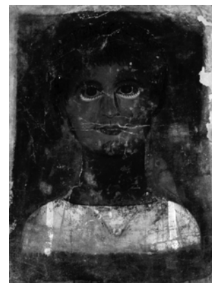
Figure 8.4 VIVL image of fig. 8.3. Camera: Nikon D90 (modified); SPEX Mini CrimeScope MCS-400 (555 nm); PECA 916 and red long pass filters (grayscale). Courtesy of the UCLA/Getty Program in Archaeological and Ethnographic Conservation
