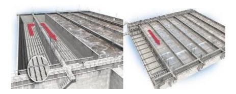
Fig 4: Aerobic process of biological wastewater treatment [8]
