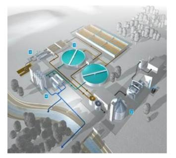
Fig. 2: Schematic presentation of water purification in MWTP (1-Mechanical preliminary treatment, 2 – Sedimentation, 3 - Sludge treatment, 4 - Microscreening, filtration) [9]
