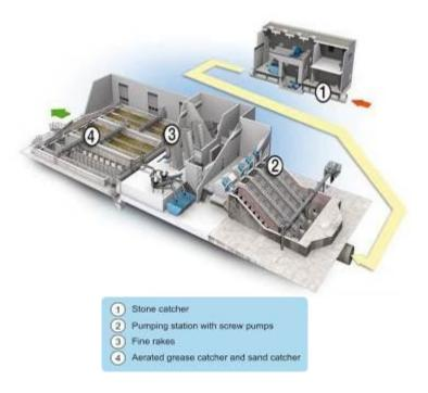
Fig. 3: Process of mechanical treatment [8]
