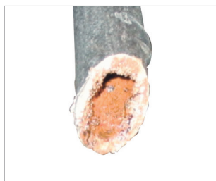
Fig. 2: Corrosion build-up in metal pipes
