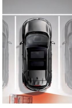
Moving Object Detection. Shift into Reverse, and the available RearView Monitor displays what's behind you. If it detects something moving by the rear of the vehicle, it gives a visual and audible alert. And whenever you want a wider rear view, just push the camera button.<sup>4, 5</sup>
