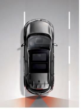
Lane Departure Warning. If Murano® detects that you're straying from your lane, the Lane Departure Warning System will give both a visual and audible alert. So smart, the system is designed to stop the warnings whenever your turn signal is engaged.3
