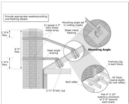
Figure V.E.2- Unreinforced masonry chimney bracing (ER).
