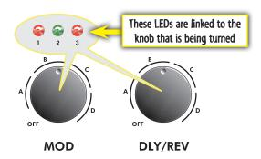
These LEDs are numbered 1, 2, 3 and correspond to the three positions within each of the selection ranges A, B, C, D on each knob. Use the LEDs to determine exactly which position the knob is pointing to, for example,  $A_1$  is shown below:
