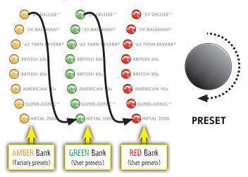
Each preset is based on one of the eight amplifier types labeled next to each of the preset LEDs. That gives you a total of three presets for each amplifier type.
