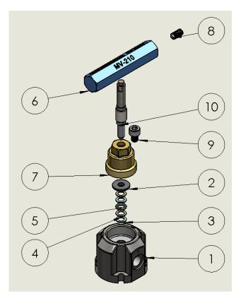
Figure 5.1: Manual Valve Exploded view
