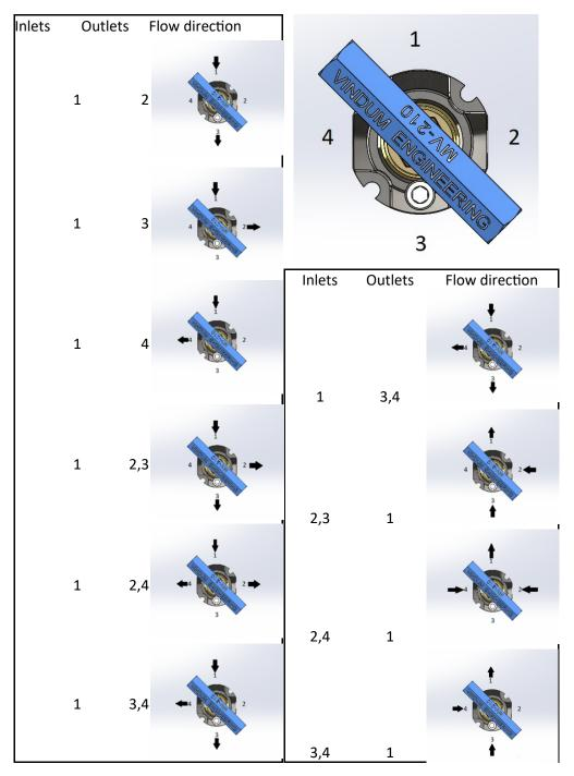
Figure 2.1: Valve options and flow directions
