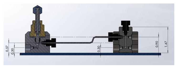
Figure 4.2: 9-way manifold dimensions.
