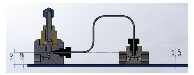
Figure 4.3: 5-way manifold dimensions
