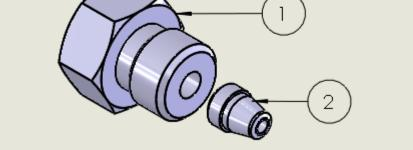
Figure 6.1: Autoclave Speedbite pressure fitting
