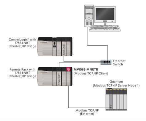
Note: The illustration does not show the required Ethernet connection for processor programming.
