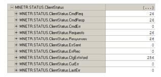
The following controller tags should increment periodically, indicating that the Modbus TCP/IP Client is continuously sending commands and receiving responses:
