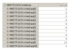
This action sends the values you entered to the **MODBUS CLIENT 0** on the MVI56E-MNETR, and then to the Quantum processor, where you will be able to see the data in Concept.
