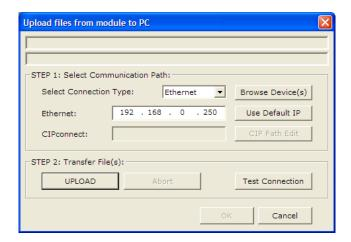
2 In the UPLOAD FILES dialog box, click BROWSE DEVICES to locate the MVI56E-MNETR module. This action opens the PROSOFT DISCOVERY SERVICE dialog box. Select the module, and then click the right mouse button to open a shortcut menu. On the shortcut menu, choose SELECT FOR PCB. This action places the module's Ethernet address in the Upload Files dialog box.
