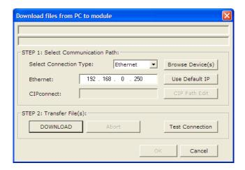
Click **TEST CONNECTION** to verify that the temporary IP address is correct.
