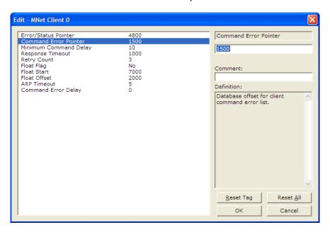
In this case, the **COMMAND ERROR POINTER** was set to 1500 and the **READ REGISTER START** to 1000. This means that (1500 – 1000 = 500); so **READDATA[500]** and **READDATA[501]** will tell you the individual status of each of the two commands issued by the module.
