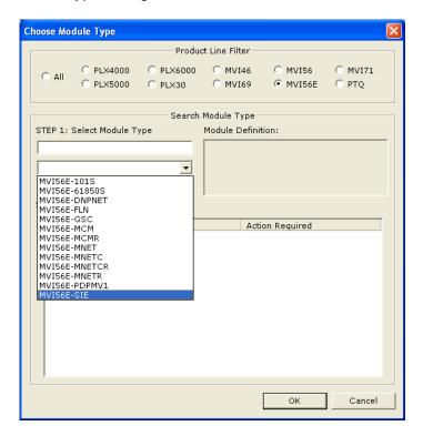
3 In the *Product Line Filter* area of the dialog box, select **MVI56E**. In the *Select Module Type* dropdown list, select **MVI56E-SIE**, and then click **OK** to save the settings and return to the *ProSoft Configuration Builder* window.
