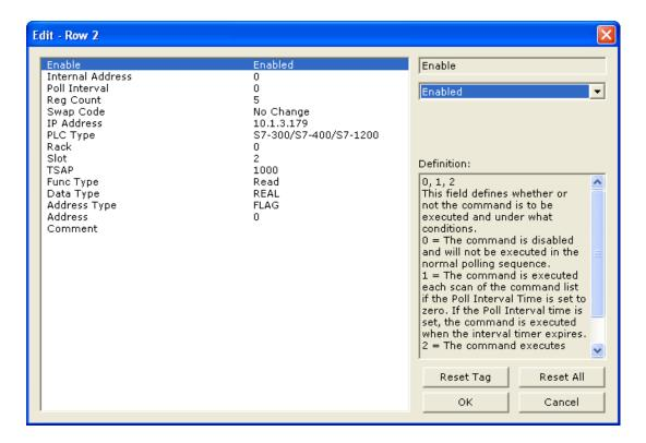
**Note:** In this example, the *Internal Address* parameter configures this command to place the data received from S7-300 processor into the first register of the module's Read Data area. The start address of the module's Read Data area is determined by the *Read Register Start* parameter in the module configuration. By default, the *Read Register Start* parameter is set to 0.
