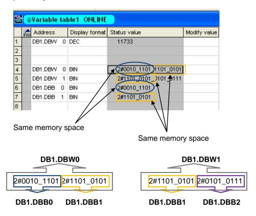
The first byte of DB1.DBW0 is the same as DB1.DBB0.
