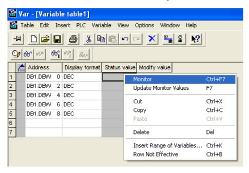
If the values from controller tags SIE.WriteData[0] through SIE.WriteData[4] were successfully transmitted, they will appear in the Status value column for addresses DB1.DBW[0] through DB1.DBW[8].
