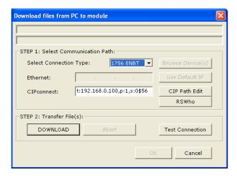
4 Click **RSWHO** to display modules on the network. The MVI56E-SIE module will automatically be identified on the network.
