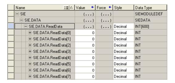
The *ReadData* array is related to the contents of the Read Data area of the module's internal database. To view the actual registers in the module's internal database, access the database display from *ProSoft Configuration Builder's Diagnostics* menu. For more information, see the section on *PCB* Diagnostics (page 122).
