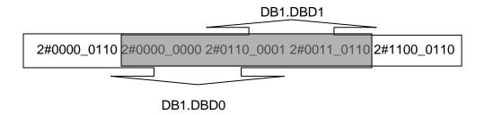
The gray area above represents the byte memory locations being overlapped when double word address is used consecutively (DB1.DBD0, DB1.DBD1, DB1.DBD2, etc).
