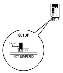
**Note:** If the module is installed in a remote rack, the Setup pins can be left jumpered. That way, the module's firmware can be updated without requiring physical access to the module.
