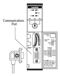
**2** Connect the straight connector end of the cable to the serial port on the computer.
