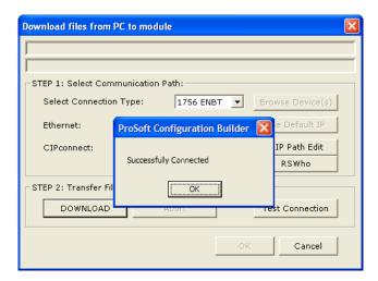
5 Click **OK** to close the Test Connection pop-up and then click **DOWNLOAD** to download the configuration files to the module through the path.
