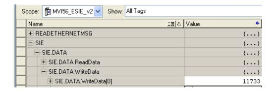
PCB screen shot showing MVI56E-SIE command to send INT data to DB1 address 0:
