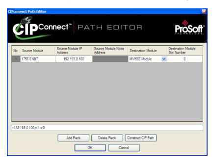
The CIPconnect Path Editor allows the path between the PC and the MVI56E-SIE module to be defined. The first connection from the PC is always a 1756-ENBT (Ethernet/IP) module.
