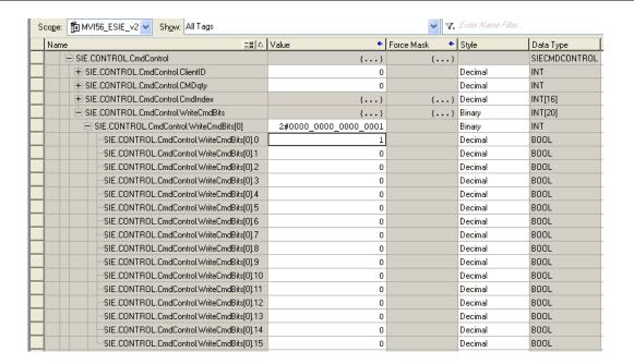
11 Check the variable table in SIMATIC Manager to see if the data transferred from the ControlLogix processor through the MVI56E-SIE module is present in the proper locations. Open SIMATIC Manager where the S7-300 processor has been set up.
