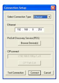
7 If the *Test Connection* is successful, click **CONNECT**. The *Diagnostics* menu will display in the *Diagnostics* window.
