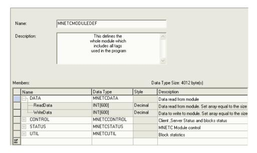
Notice that these UDTs are the data types used to declare the SIE.DATA.ReadData and SIE.DATA.WriteData controller tag arrays.
