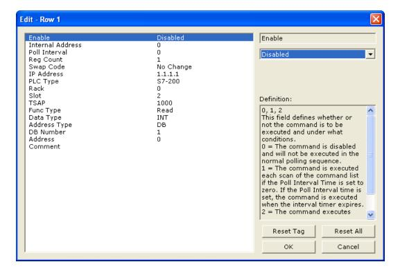
5 Select each parameter and edit its value according to the table below. (Use the IP address applicable to your network.)
