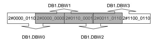
The gray area above represents the byte memory locations being overlapped when word address is used consecutively (DB1.DBW0, DB1.DBW1, DB1.DBW2, etc).
