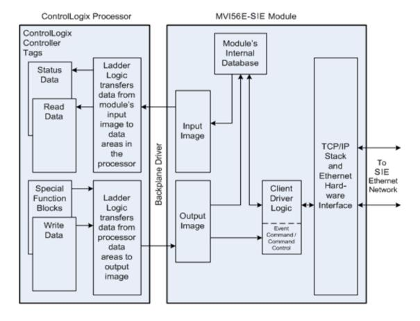
All data transferred between the module and the processor over the backplane is through the input and output images. Ladder logic must be written in the ControlLogix processor to interface the input and output image data with data defined in the controller tags. All data used by the module is stored in its internal database. This database is defined as a data table with addresses from 0 to 4999
