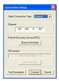
You can also use CIPconnect<sup>®</sup> to connect to the module through a 1756-ENBT card. Refer to Using CIPconnect to Connect to the Module (92) for information on how to construct a CIP path.
