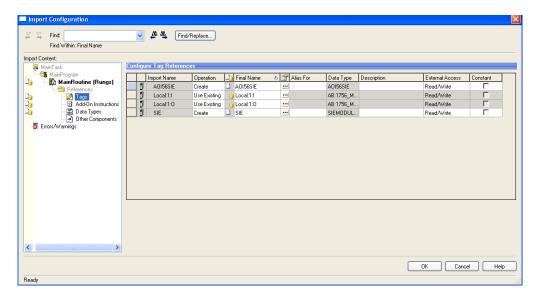
5 If the module is being used in a different slot (or remote rack), select the correct connection input and output variables that define the path to the module. If the module is located in Slot 1 of the local rack, this step is not required.
