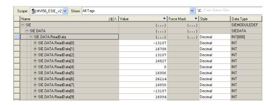
13 To display the data in floating-point format, copy it into an array with a REAL data type. Click the **EDIT TAGS** tab at the bottom of the *Controller Tags* window and enter a name for the array (in this example, **REALDATA**). In the *Data Type* column, enter **REAL[5]**.
