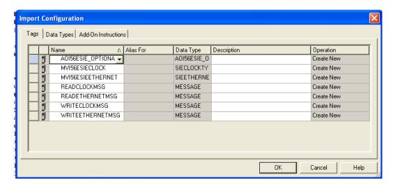
The Add-On Instruction will be now visible in the ladder logic. Observe that the procedure has also imported data types and controller tags associated with the Add-On Instruction.
