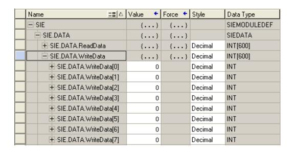
The *WriteData* array is related to the contents of the Write Data area of the module's internal database. To view the actual registers in the module's internal database, access the database display from *ProSoft Configuration Builder's Diagnostics* menu. For more information, see the section on *PCB* Diagnostics (page 122).
