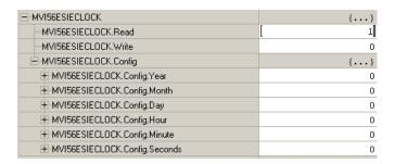
The bit will be automatically reset and the current clock value will be copied to MVI56ESIECLOCK.Config controller tag as follows.
