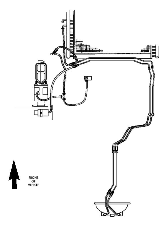
REAR DIFFERENTIAL COOLER INSTALLED
