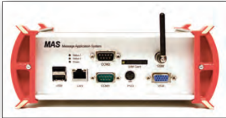
Figure 2. Comron alarm server features a wide range of interfaces, via which incoming messages and alerts can be distributed to other devices taking different priorities, dates, schedules and requirements into account.
