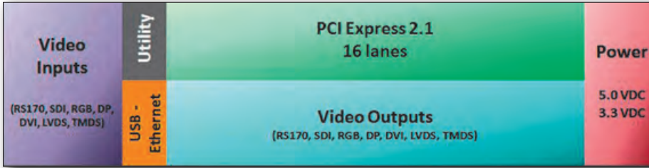
Figure 1. The MXC pinout is specifically geared towards a wide variety of video input and output formats, with 16 lanes of PCIe to support data communication.
