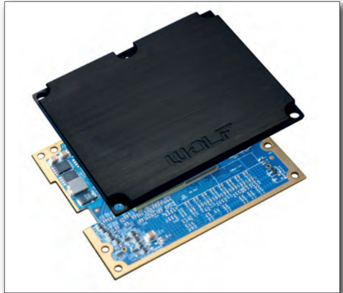
Figure 4. The MXC module seen from above, and with the heat shield shown detached from the board it protects. The heat shield allows the use of reliable conduction-cooling techniques.
