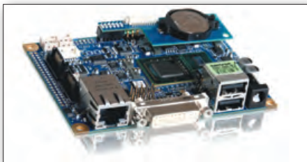
Figure 3. Kontron Pico-ITX Motherboard pITX-SP integrates Intel Atom processors and standard interfaces in a tiny footprint.
