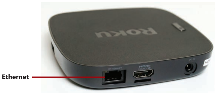
The Ethernet connection on the back of the Roku Ultra player. (Photo courtesy Roku, www.roku.com .)
