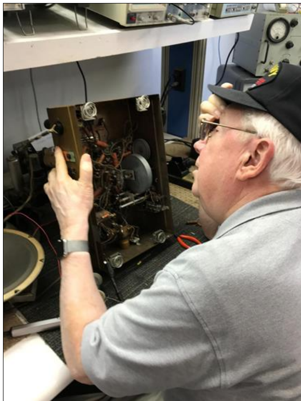
Jim Rogers working on a Zenith Console radio with bad wiring.
