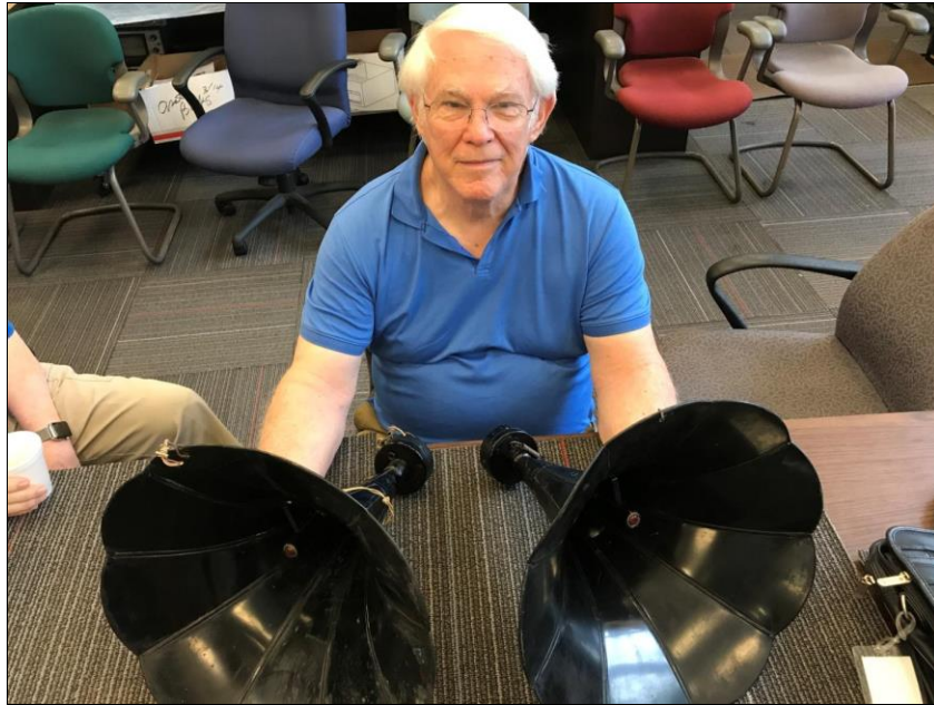
Mack White with two early Western Electric Model 360 Horn microphones (and they work). Note the "on the air" red lights inside each microphone.
