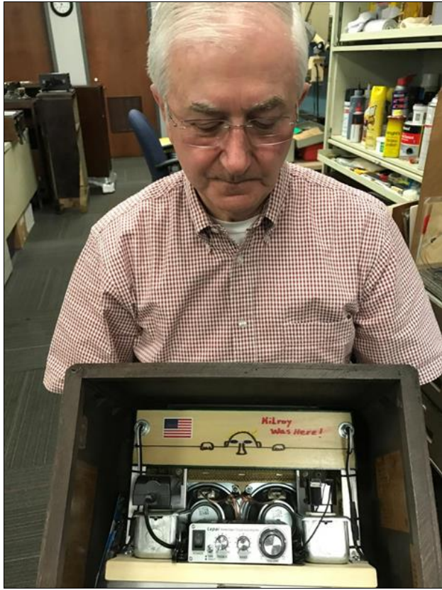
Frank Parker restored the exterior and replaced the electronics inside with dual speakers and a blue tooth receiver and amplifier.
