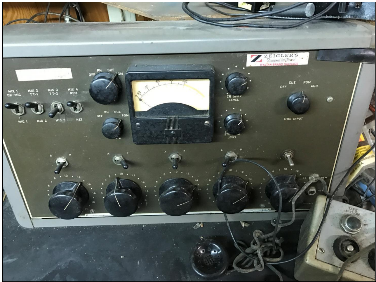
The main studio mixer used for mixing the live broadcasts each day.
