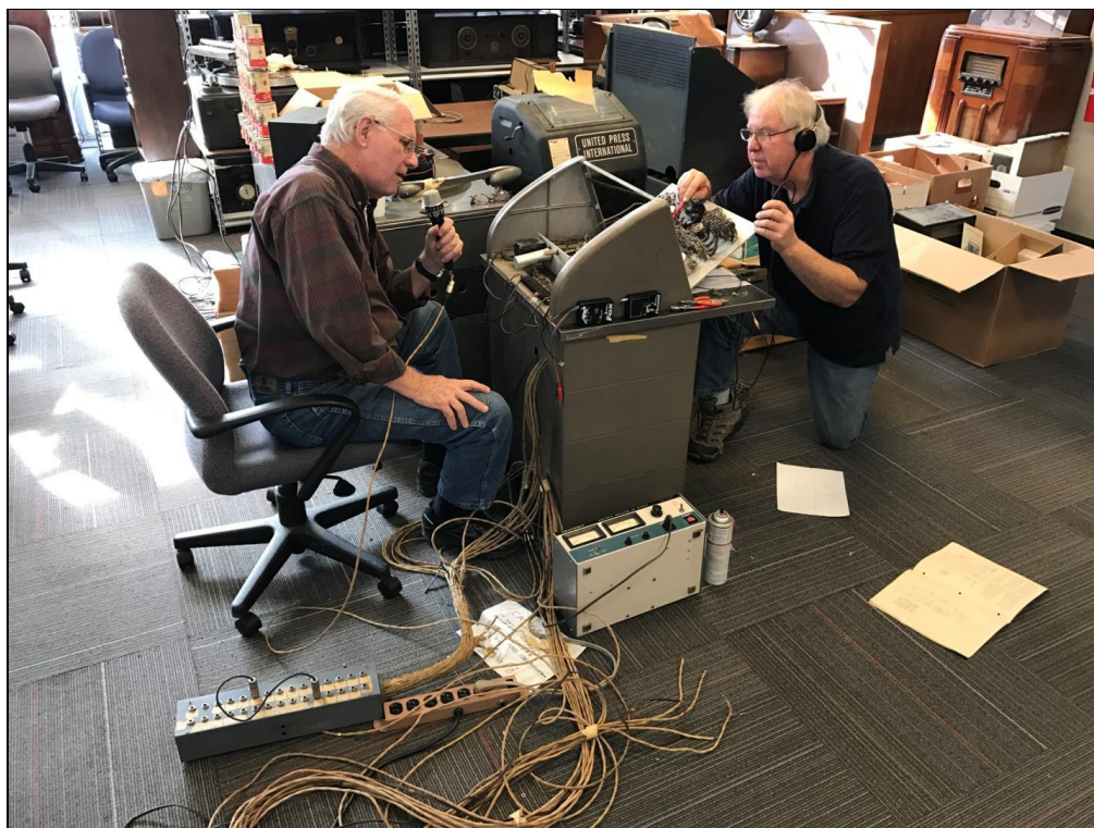
Ed Boutwell and Jim Cawthon ringing out the multiple circuits in the main mixer.
