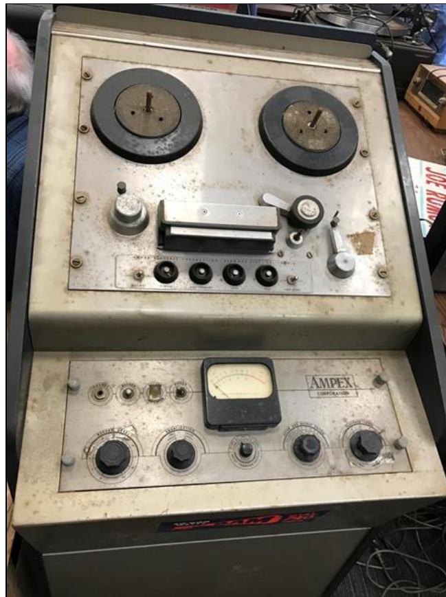
1950's Ampex Series 350 Reel to Reel Recorder with Electronics mounted in a Console.
