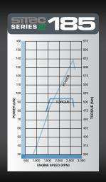
SiTEC Series III 185 produces 139kW power and 510Nm torque and is standard on NQR models.
