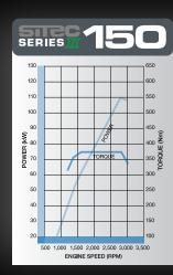
SiTEC Series III 150 produces 110kW power and 375Nm torque and is standard on NLR, NLS and NNR models.
