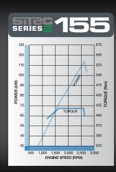
SiTEC Series III 155 produces 114kW power and 419Nm torque and is standard on NPR and NPS models.
