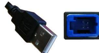
NV-NIUSB2 USB Port Retention Harness - Select 2010-Up Nissan With 4-PIN
