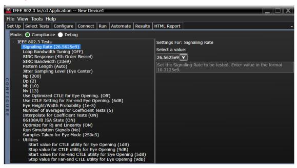
Customize parameters that are specific to your setup, such as signaling rate and CTLE setting. Use default values or enter your own settings including number of waveforms taken, type of pattern, and pattern symbol length. Choose Normal mode to test within limits or choose Debug mode to test to your custom limits and adjust other test parameters. Choose Your Tests
