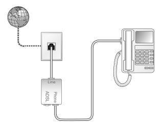
2. Use the included phone cable with RJ-11 jacks to connect the ADSL port (A) of the wireless modem router to the ADSL port (B) of the two-line ADSL microfilter.
