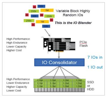
Figure 15: IO Consolidation write de-amplification.
