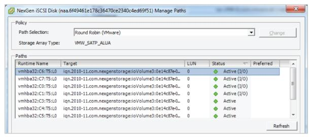
Figure 138: MPIO ALUA setup on ESX host
