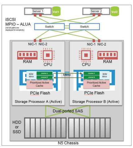
Figure 127: Pivot3 N5 Active-Active PCIe flash Architecture Diagram.
