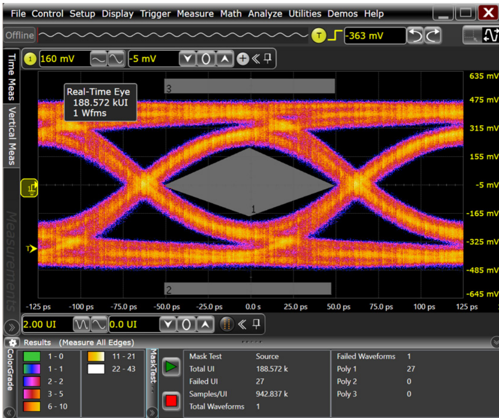
Figure 21. The E2688A and N5461B applications allow for the equalization of impaired 8 and 16 Gb/s signals so a clock can be recovered and mask testing can be performed on your waveforms.
