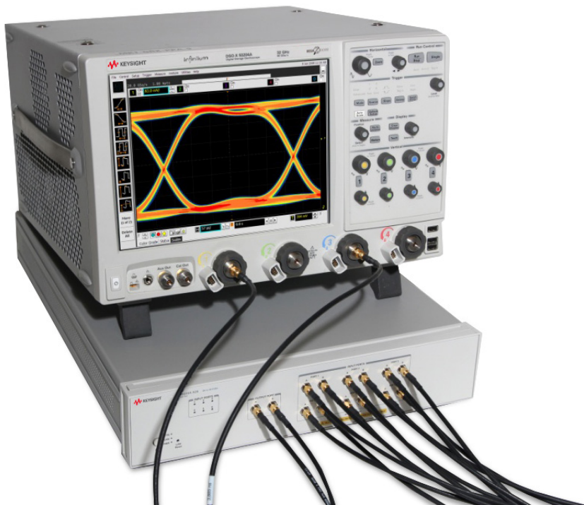
Figure 17. Automated testing for multi-lane digital bus interface through switching solution.
