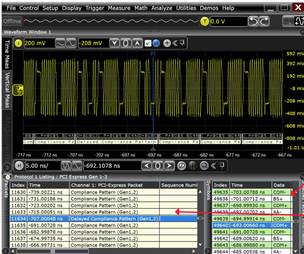
Figure 20. The N5463A provides 8b/10b and 128b/130b decode below.
