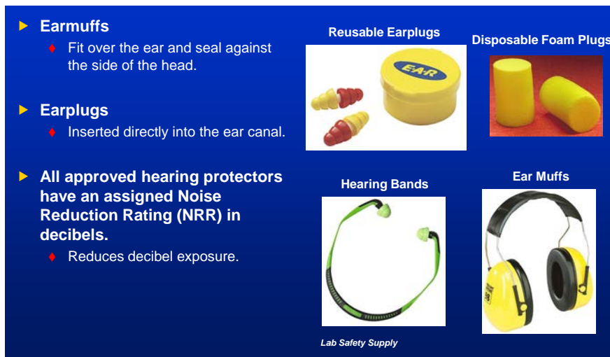
Figure 94. Hearing protection should be used whenever using machinery or power tools with noise levels exceeding 85 dB.
