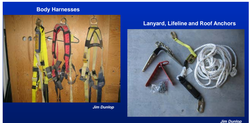
Figure 87. A personal fall arrest system (PFAS) consists of an anchorage and connectors, a body harness, and a lanyard/deceleration device.
