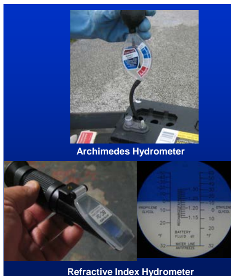
Figure 117. Hydrometers measure electrolyte specific gravity (SG).
