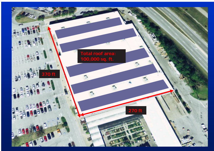
Figure 7. For a power density of 10 watts per square foot, a 500 kW PV array can be installed in a 50,000 square foot area.
