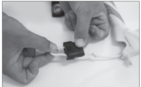
D) Pull the leader line out through the bottom of the adjusting cavity (3).
