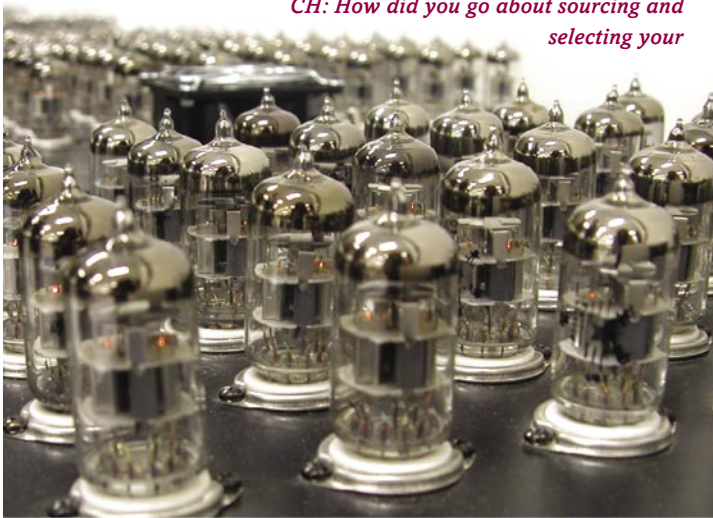
All the tubes used in the mics are 'burnt in' – where each valve is put under a load to determine which will fail.
