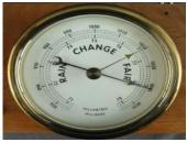
The Isobar Map's data is collected by reading a barometer.
