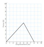
13. The force as a function of displacement of a moving object is presented by the graph. How much work is done when the object moves from 5 m to 8 m?
