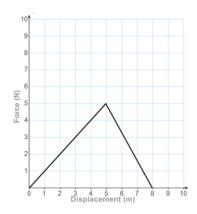
12. The force as a function of displacement of a moving object is presented by the graph. How much work is done when the object moves from 0 m to 5 m?
