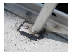
The stanchions are attached to the toerail; each was physically tested and found to be secure apart from those around the port and starboard boarding gates. The forward port gate stanchion was loose and the feet for the aft one did not lie fair to the deck. On the starboard side the foot for the forward gate stanchion has been refastened to the deck, though it still does not lie fair, see photo. The stanchion itself was more secure than the equivalent one on the port side.
