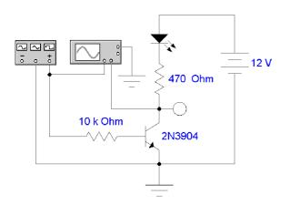
Figure 1.2: Transistor as a switch
