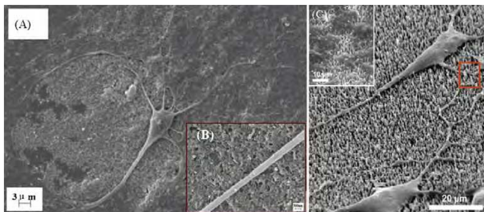
Fig. 2. a Neonatal hippocampal neurons adhering on purified multi-walled carbon nanotubes-coated glass substrates, showing extended neuritis after 8 days of culture; (B) single neurite in close contact to carbon nanotubes; (C) PC12 neural cells grown on vertically aligned carbon nanotubes coated with polypyrrole. Images from (Zhang & Webster, 2009). Reproduced with permission from Elsevier.
