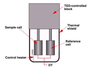
**Figure 4** Nano ITC measuring unit.
