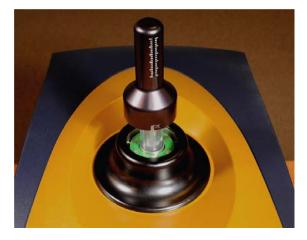
Figure 16 Inserting the buret into the calorimeter.
