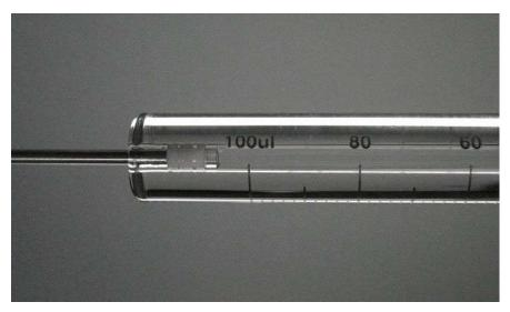
Figure 13 Syringe with air gap.
