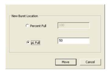
As an alternative, the desired position can be entered as a percent of the full capacity.
