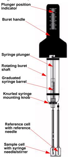
**Figure 6** Orientation of buret, syringe, needles, and cells during experiments.
