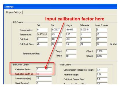
Figure 10 Calibration factor location.
