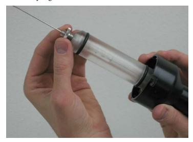
Figure 15 Tightening the syringe into place.
