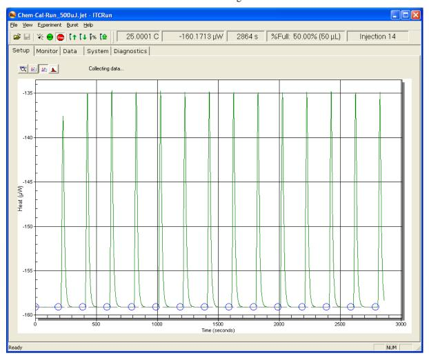
**Figure 9** Example of successful calibration.
