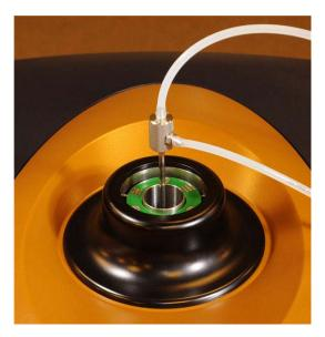
Figure 18 Tubing connected to cleaning tool.
