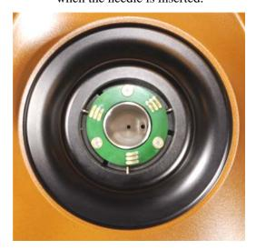
Figure 12 Sample (center) and reference (right) cell access tubes.
