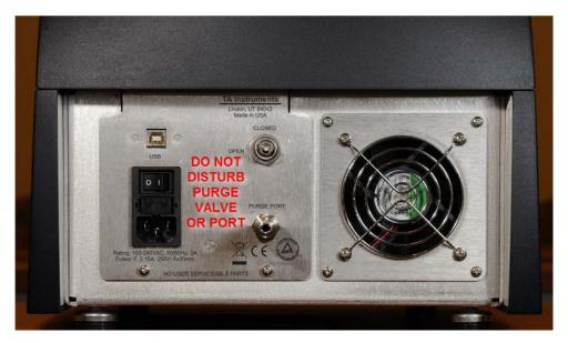
Figure 21 Location of purge valve and port on rear of instrument.
