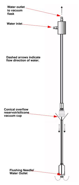
Figure 19 Side view of cleaning tool in sample cell.
