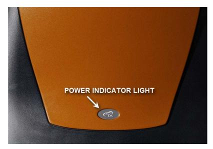
Figure 8 LED location on Nano ITC Low Volume instrument.
