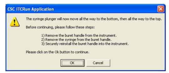
After the buret drive stops moving, it will be located at the top position and the buret position will be reported as 100% on the top of the Nano ITC screen.
