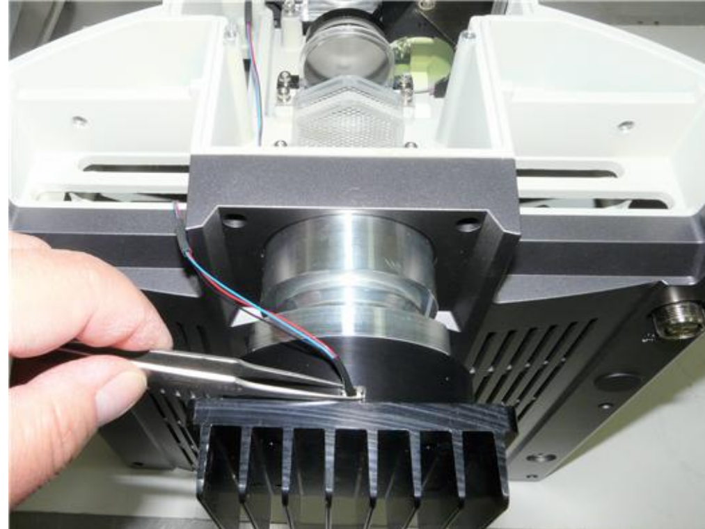
Photo 29. Plug the pot cable in.
