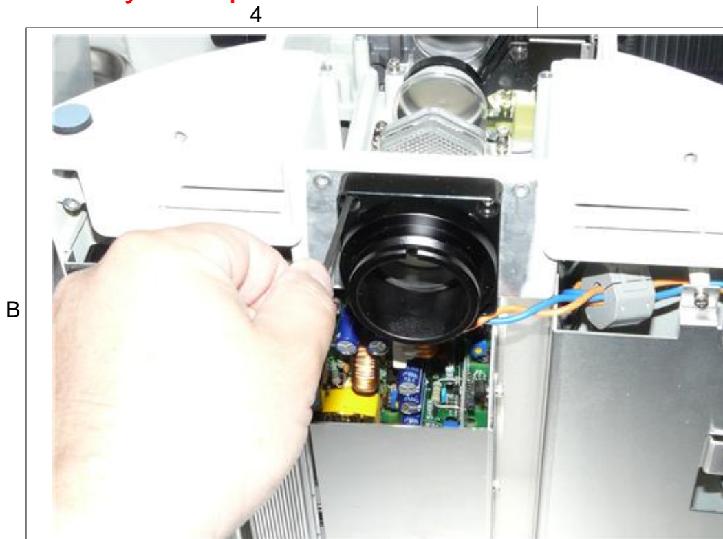
Photo 19. Remove original illuminator adapter.
