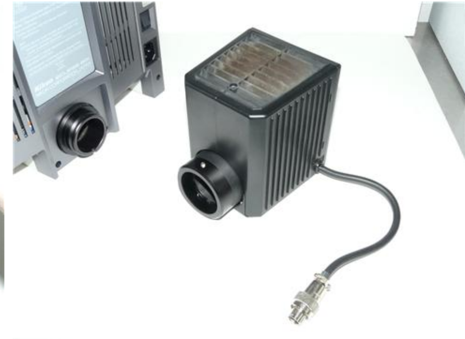
Photo 3. Remove the original lamp house.
