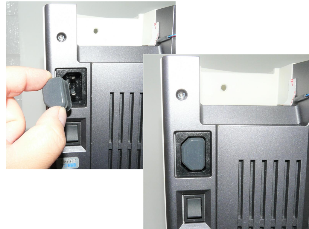
Photo 33. Install PN 10736 rubber plug in the AC receptacle.
