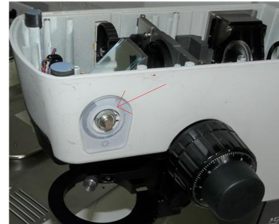
Photo 6. Remove hex nut (red arrow) by using 12mm hex socket.
