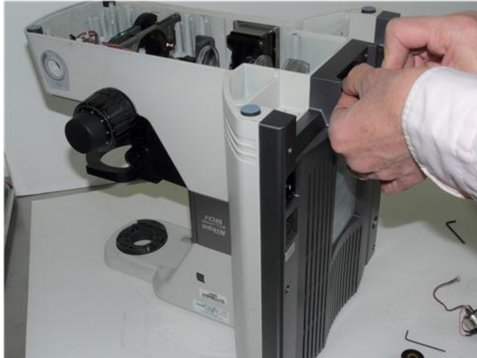
Photo 11. Remove back cover by loosening screws.
