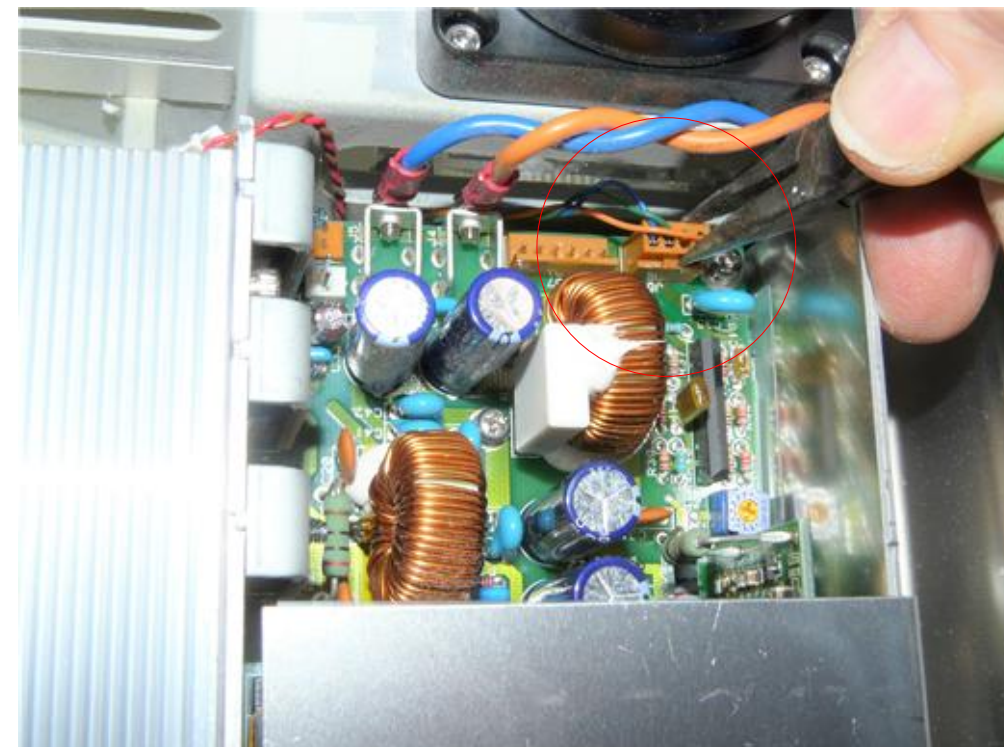
Photo 15. Disconnect orange color connector from circuit board.
