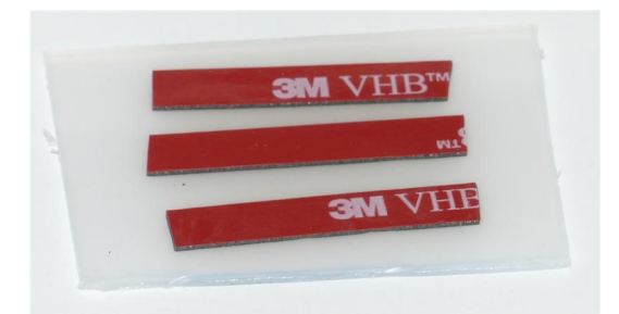
3M VHB tape to secure pot cable
