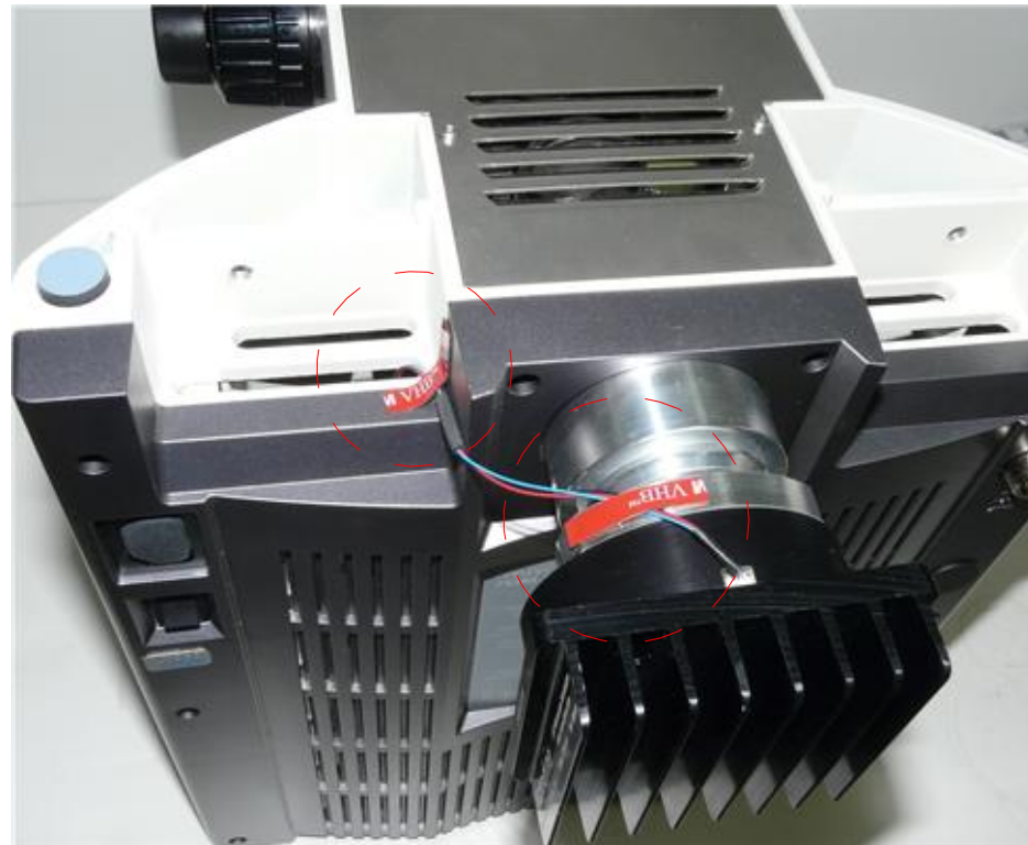
Photo 32. Secure the wire using provided 3M VHB tape if needed.
