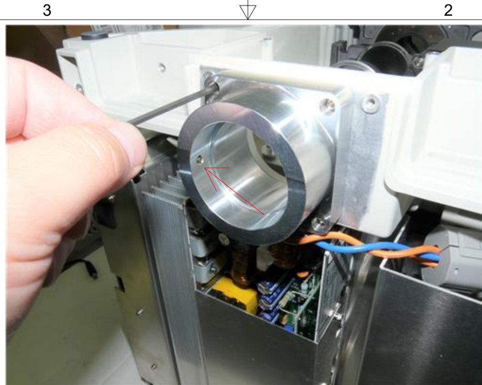
Photo 20. Install Nanodyne adapter.
