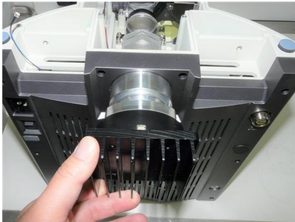
Photo 27. Insert Nanodyne illuminator to the port.
