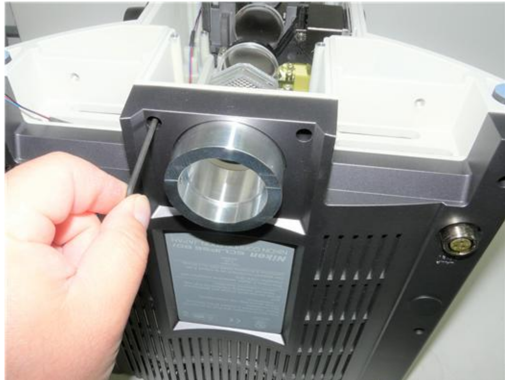
Photo 26. Re-install the back cover.
