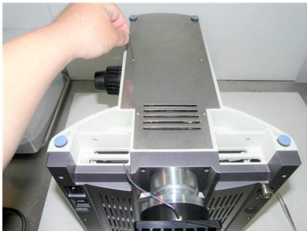
Photo 31. Screw the bottom cover back in place.
