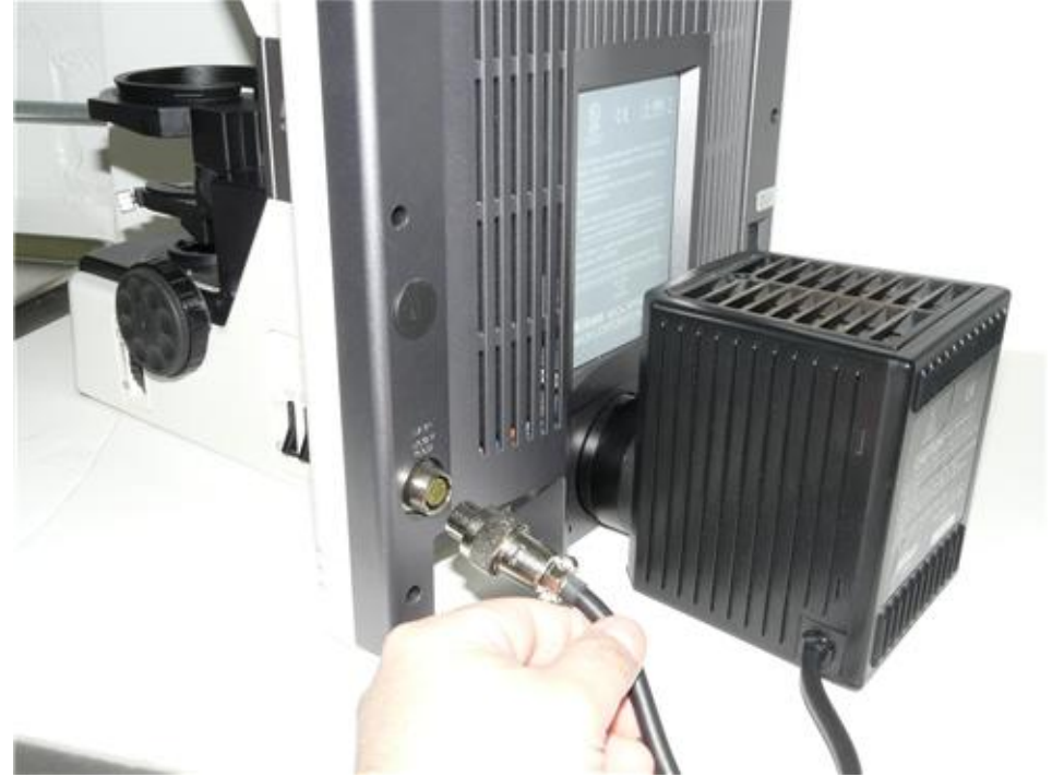
Photo 1. Unplug the original lamp cable.
