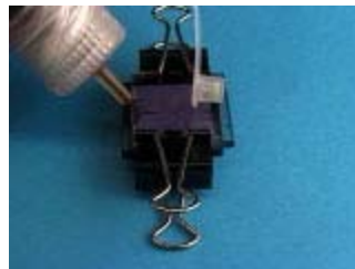
Dope with \text{KI}_3 solution
