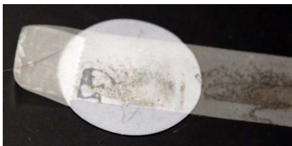
Transfer graphite to Scotch tape
