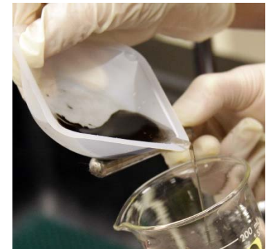
Rinse with water and tetramethylammonium hydroxide
