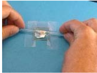
Coat surface conducting glass
