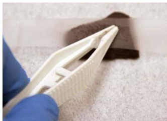
Transfer graphite to Scotch tape
