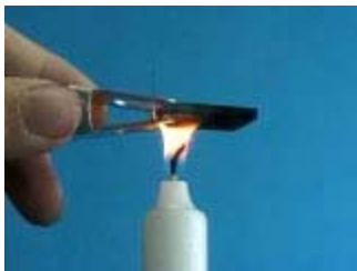
Coat 2 nd piece of glass with carbon
