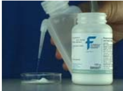
Prepare polyvinylalcohol solution
