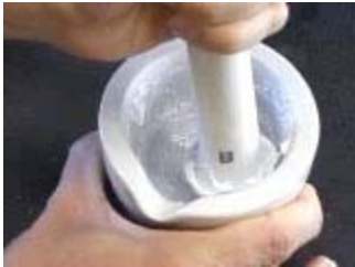
Grind nanocrystalline \text{TiO}_2 with dilute acetic acid
