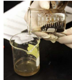
Decant liquid and transfer solid to a weighing boat
