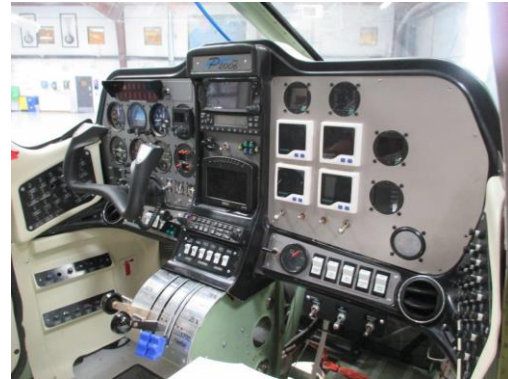
Figure 2.2-3: X-57 cockpit includes new instrument panel configured to manage the electric powertrain
