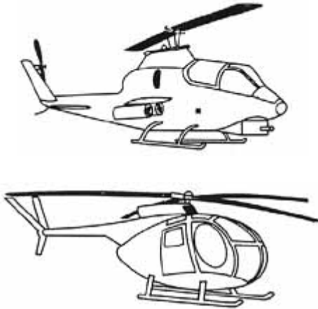
(a) Bell AH-1G Huey Cobra. Two-bladed. (b) Hughes OH-6A. Four-bladed.
