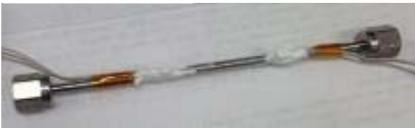
Figure 4. Mounted RTDs on Tubes #1, #2, and #3.
