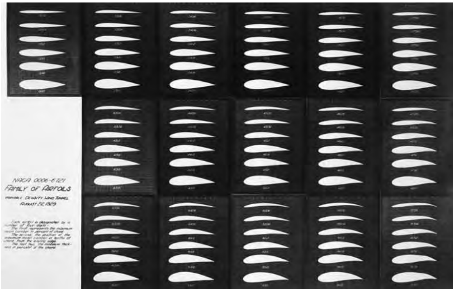
Figure 2: NACA 4 Digit Airfoils. NASA Image EL-2003-00333
