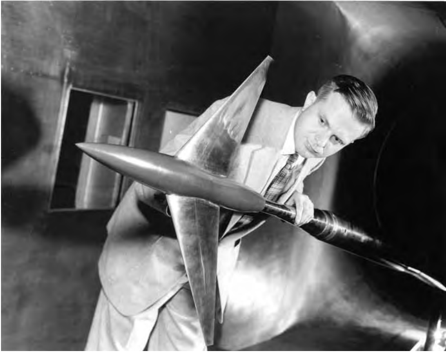
Figure 12: Richard T. Whitcomb with an area-ruled swept-wing research model. NASA Image L-89119
