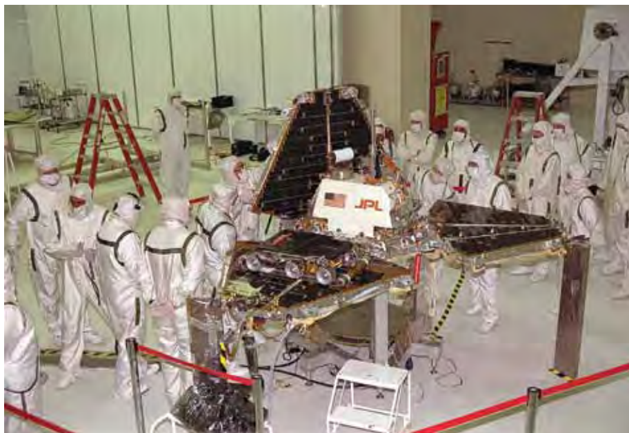
Figure 1: Strong in-house technical capability formed the basis for NASA's original organization culture. Here, Jet Propulsion Laboratory employees close the metal petals of the Pathfinder lander dispatched to Mars in 1996. The Sojourner small rover is visible on one of the three petals. NASA Image 96PC-1130
