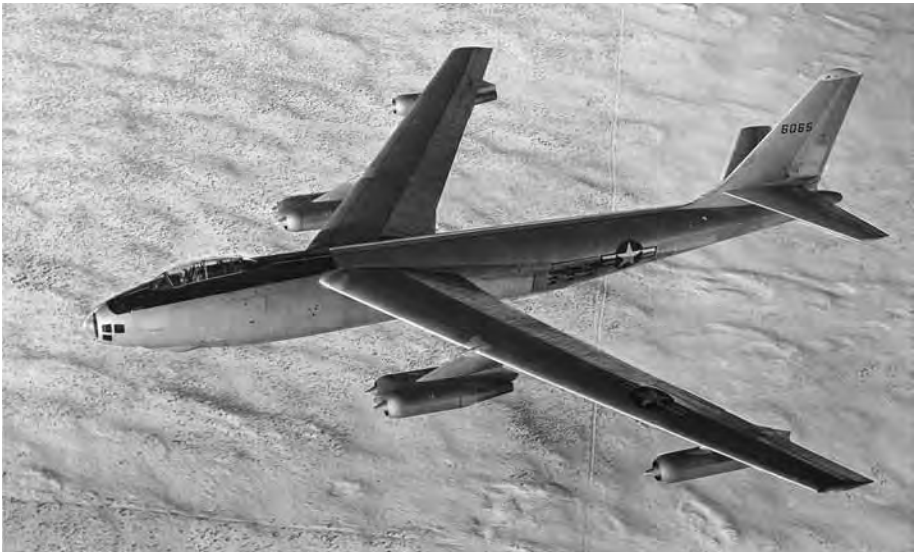
Figure 10: The Boeing XB-47, which introduced the design standard of wing-mounted engine pods combined with a swept-wing platform. Air Force Flight Test Center History Office
