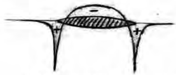
SECTION B-B ENLARGED, SHOWING PRESSURE DISTRIBUTION
