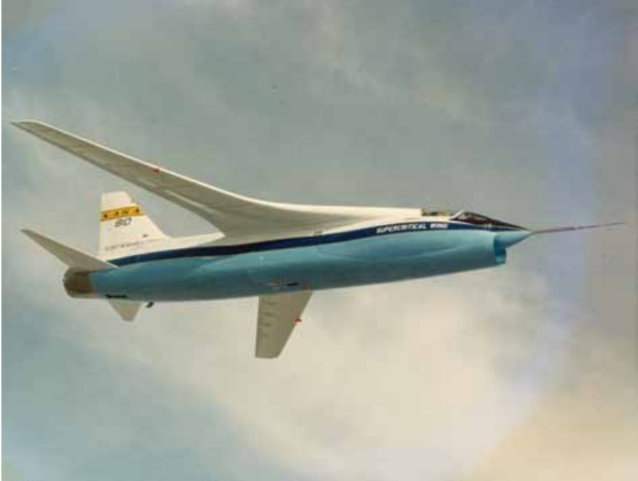
Figure 15: The NASA F-8 SCW test bed, with a high-aspect-ratio transport-optimized wing planform. NASA Image ECN 3468
