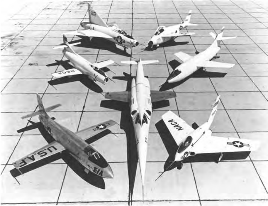
Figure 11: The “Round One” Research Aircraft, 1953. From the lower left are the Bell X-1A, Douglas D-558-1, Convair XF-92A, Bell X-5, Douglas D-558-2, and Northrop X-4. At the center is the Douglas X-3. HSFS Image E-2889
