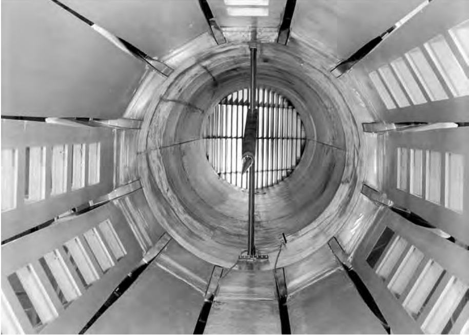
Figure 3: The Langley 8-Foot High-Speed Tunnel. The slotted walls of the test section permitted accurate testing at transonic speeds. NASA Image EL-2003-00280
