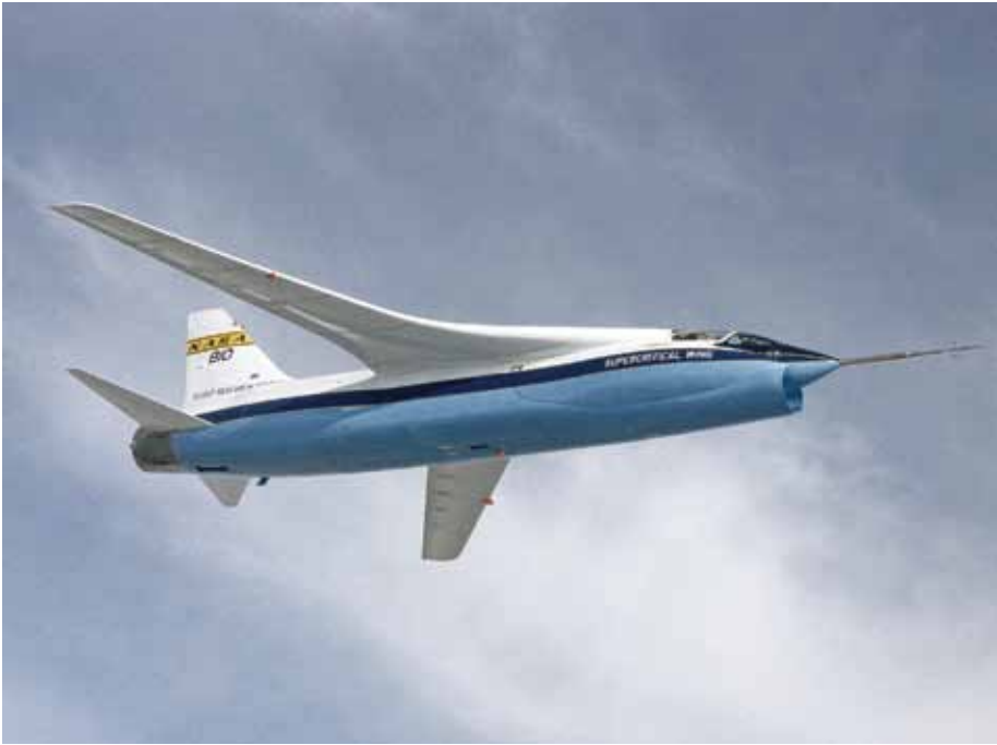
Figure 2: F-8 supercritical airfoil. NASA Image EC73-3468
