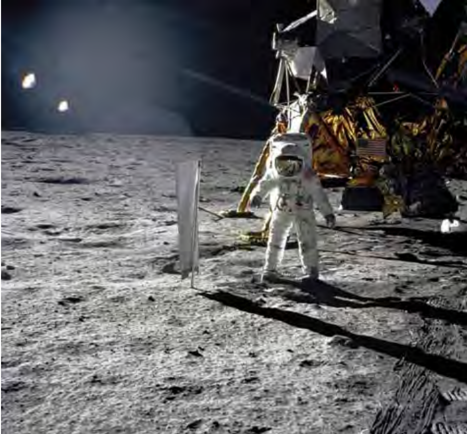
Figure 1: Astronaut Edwin E. “Buzz” Aldrin, Jr., Lunar Module pilot during the Apollo 11 extravehicular activity (EVA) on the lunar surface. In the right background is the Lunar Module Eagle. On Aldrin’s right is the Solar Wind Composition Experiment already deployed. This photograph was taken by Neil A. Armstrong with a 70-millimeter lunar surface camera. NASA Image AS11-40-5873
