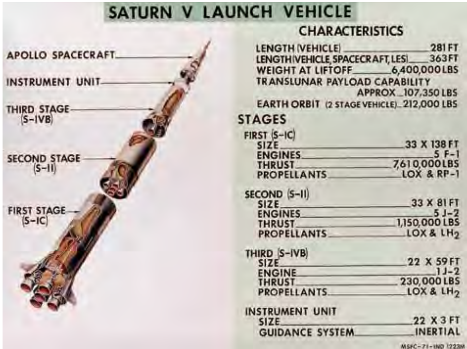
Figure 2: Diagram of a Saturn V launch vehicle's components and characteristics. NASA
