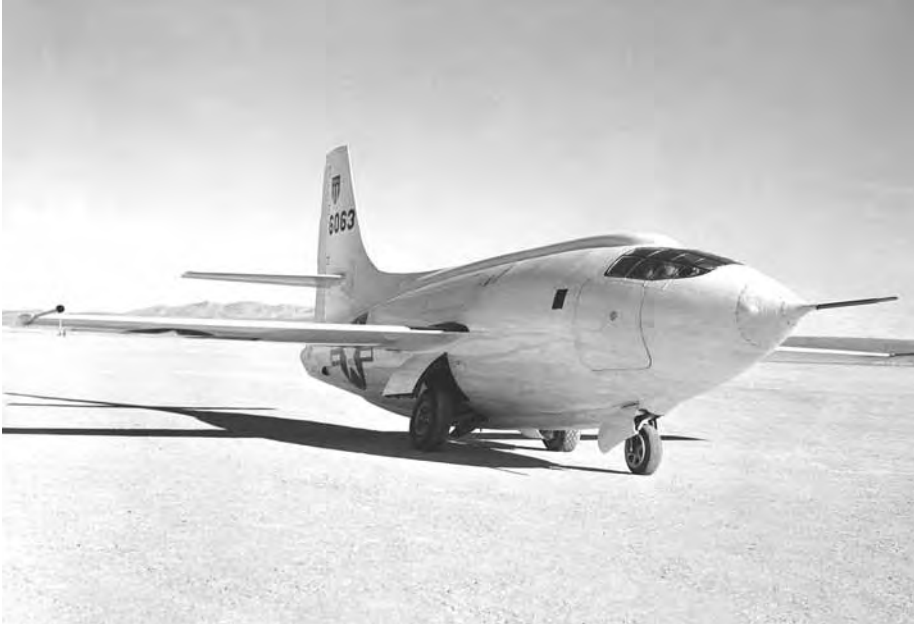
Figure 4: The Air Force-sponsored, rocket-powered Bell XS-1 (X-1), whose fuselage shape copied the .50 caliber machine gun bullet. This is the second X-1 (AAF 46-063), eventually modified as the Mach 2+ Bell X-1E. NASA Image E49-001
