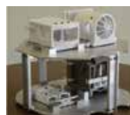
NASA Langley's Mars Packing Efficiency Payload which is testing the development of deployable Mars rover packing concepts to improve lander packing efficiency and aerodynamic stability during aerocapture and EDL.
