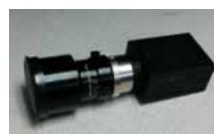
Low cost star tracker designed to provide arcsecond level accuracy using commercial off the shelf components and internal labor.
