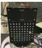
Orbital ATK's LEO-2 CubeSat experiment for testing ultra-lightweight advanced materials including carbon nanotube (CNT) materials for structures and additive manufacturing.
