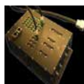
Tyvak's Nano-Launch Vehicle Avionics (NLVA) System which provides complete GNC functionality, analog sensor polling, power and telemetry distribution, and GPS metric tracking in the industry's smallest form factor. Developed under a NASA Phase II SBIR from Kennedy Space Center that ended in April 2016.
