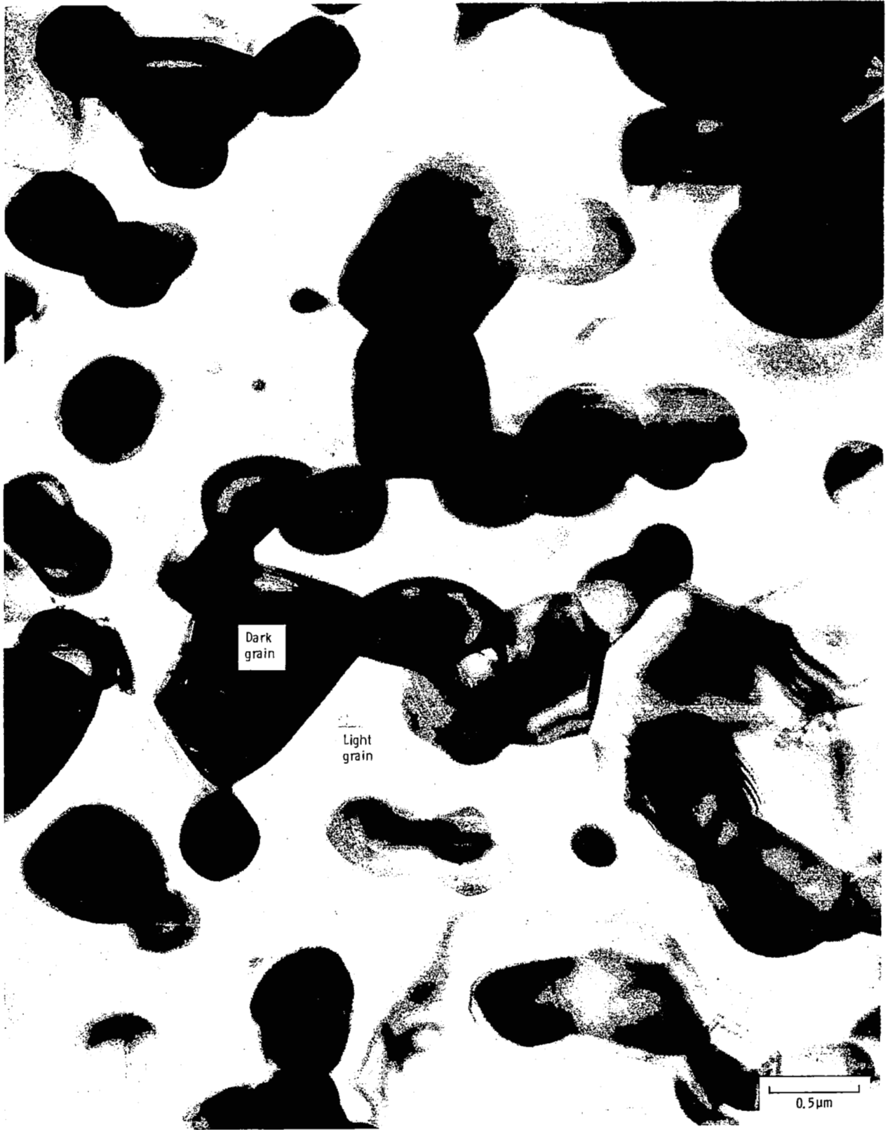
Figure 6. - Typical microstructure of a metallic glass ( \text{Fe}_{67}\text{Co}_{18}\text{B}_{14}\text{Si}_1 ) heated to 750^\circ\text{C} in vacuum (10 nPa).
