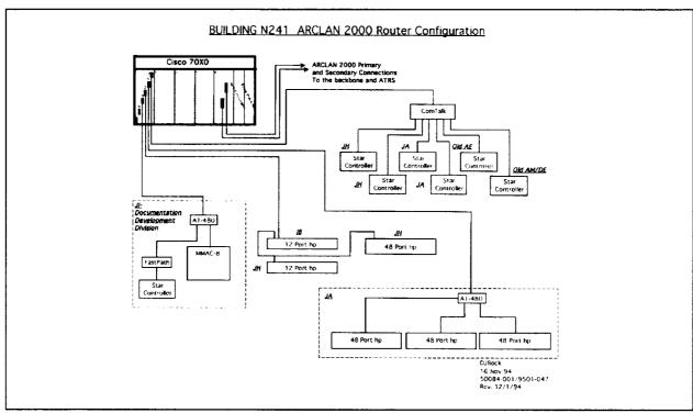
Figure 3 - 7. ARC EDD interface to ARCLAN 2000.
