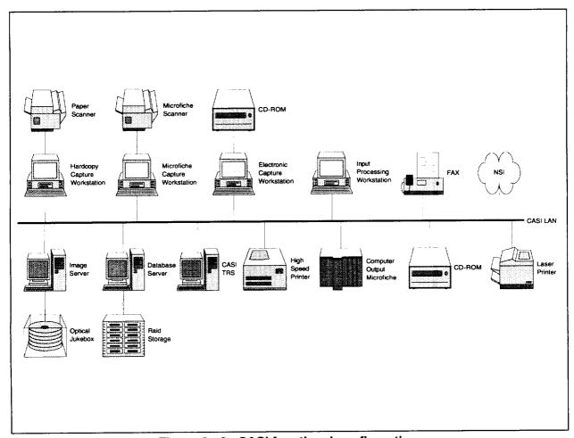
Figure 3 - 9. CASI functional configuration.
