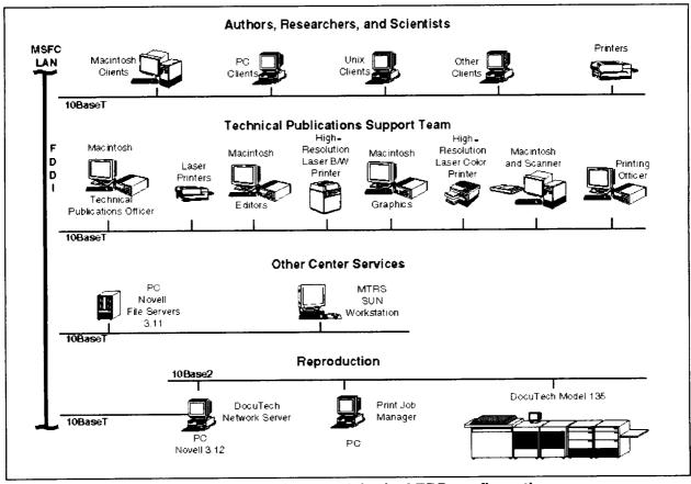
Figure 3 - 13. MSFC network logical EDP configuration.
