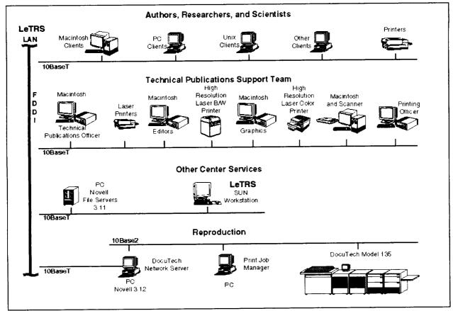
Figure 3 - 5. LeRC network logical EDP configuration.
