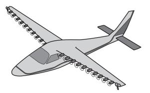
The aeroplane is powered by 22 motor-driven propellers that each supply 18 kW.
