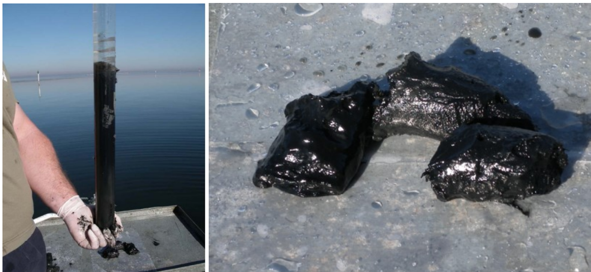
Figure 5.3 Black oily appearance of MBO gel collected from the Peel region, Western Australia.
