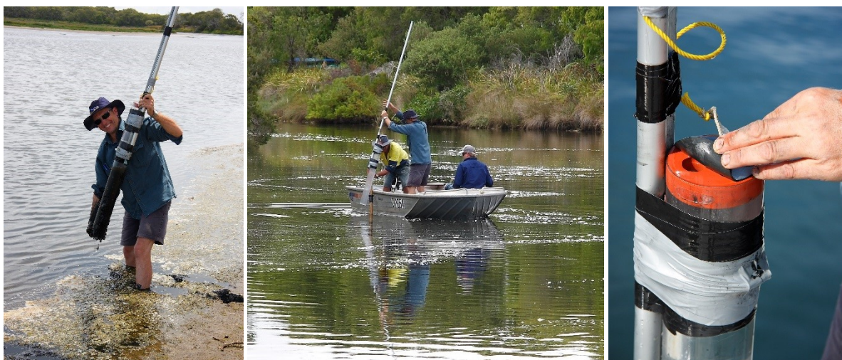
Figure 6.2 Sampling MBOs using a sediment coring device.
