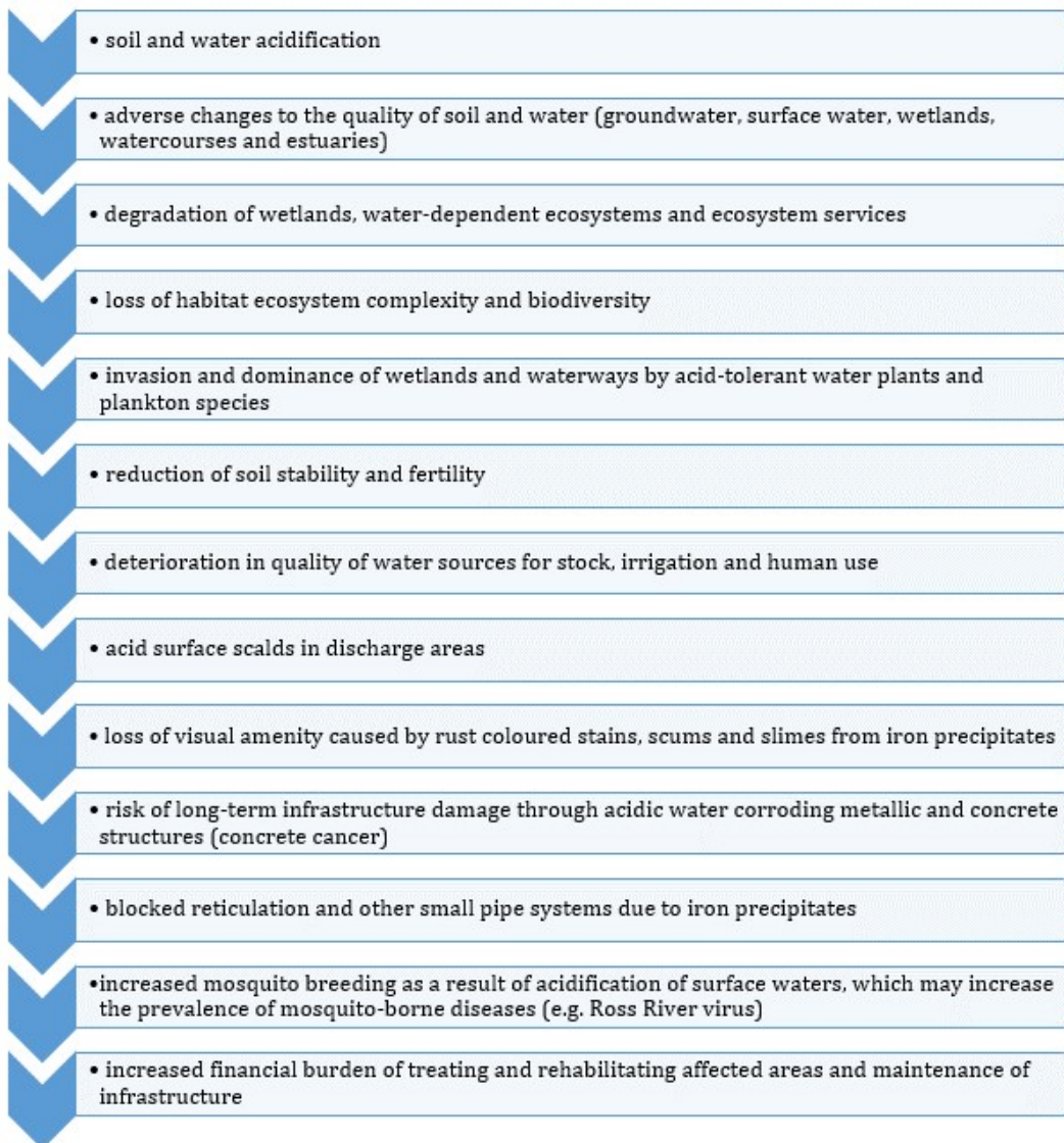
Figure 2.3 Potential impacts due to the disturbance of ASS materials.
