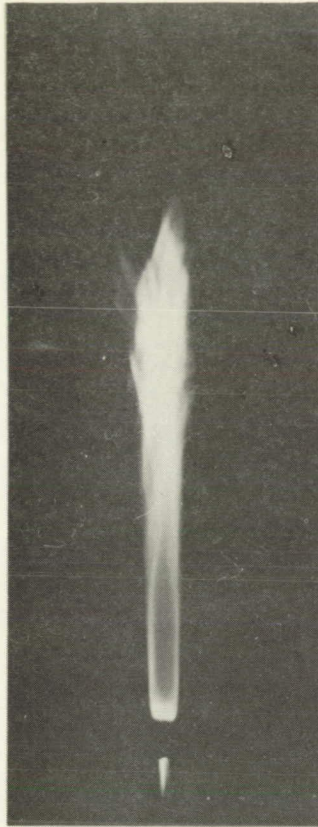
(b) Suspended flame; turbulent flow; Reynolds number, 3770; fuel-air ratio, 0.183.
