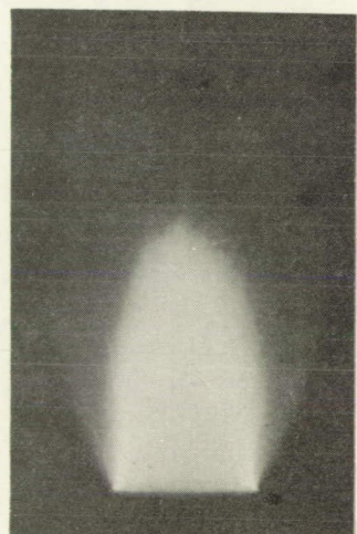
(f) Seated flame; turbulent flow; Reynolds number, 3770; fuel-air ratio, stoichiometric.
