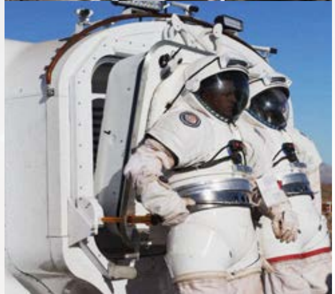
The Desert RATS analog mission tested a suitport prototype. Top, a crewmember enters the suitport from inside a prototype MMSEV, and bottom, now outside the vehicle, he detaches the suit and life support pack from the MMSEV to begin an EVA.
