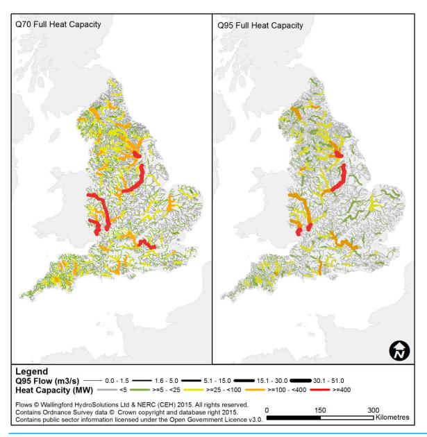
Figure 17 Comparison of heat capacity estimated using Q70 and Q95 winter flow
