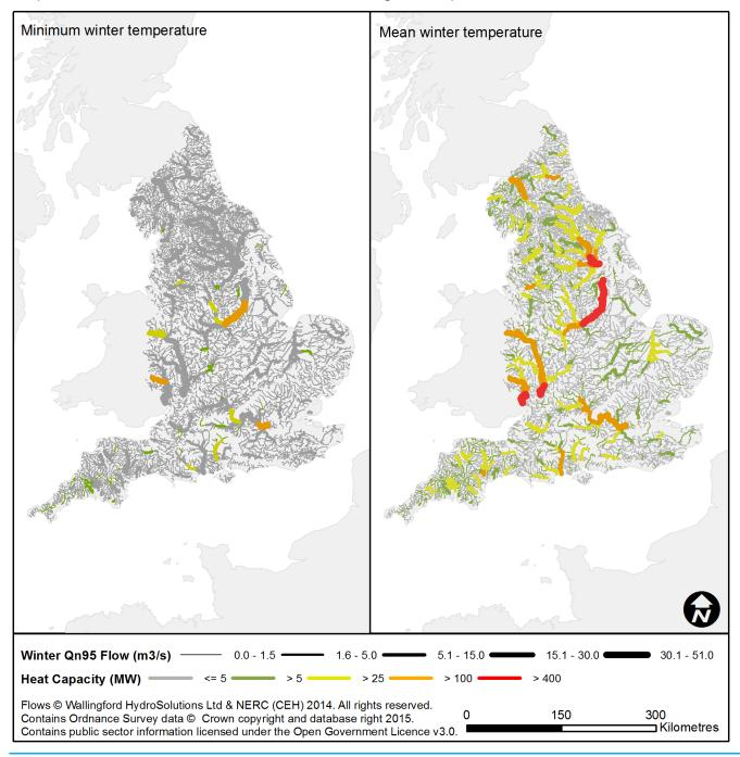
Figure 16 Comparison of heat capacity estimated using minimum and mean winter temperatures
