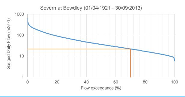
Figure 1 Example flow duration curve in blue, the orange line explains Q70 as the gauged daily flow equalled or exceeded 70% of the time.
