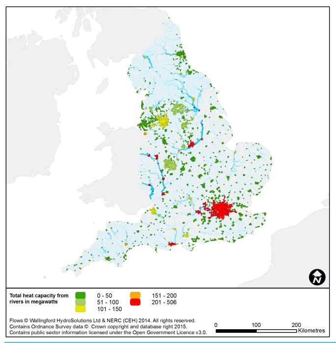
Figure 14 Total heat capacity from rivers in megawatts for urban areas
