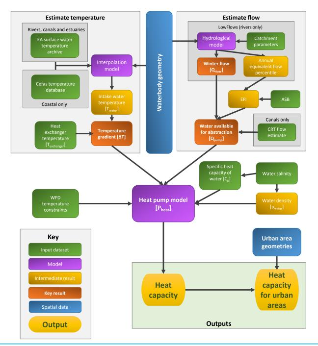
Figure 20 Flowchart illustrating relationships between key input data, algorithms and results
