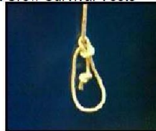
Bowline with an Overhand Knot
