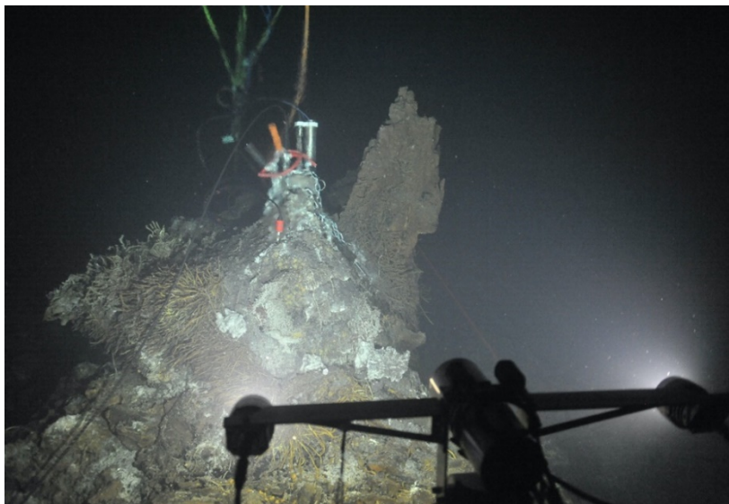
The Regional Cabled Array cabled digital still camera, redeployed in 2015 by the Canadian ROV ROPOS, lights up the active hydrothermal vent called El Gordo in the international District Hydrothermal Field, located at the summit of Axial Seamount nearly a mile beneath the ocean surface. Credit: UW/NSF-OOI/CSSF.
