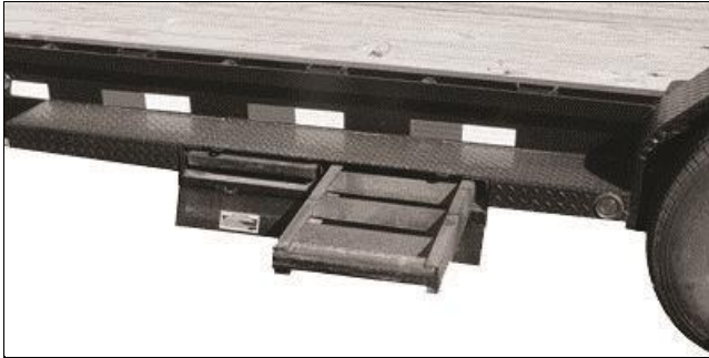
Side Storage Position Ramps
