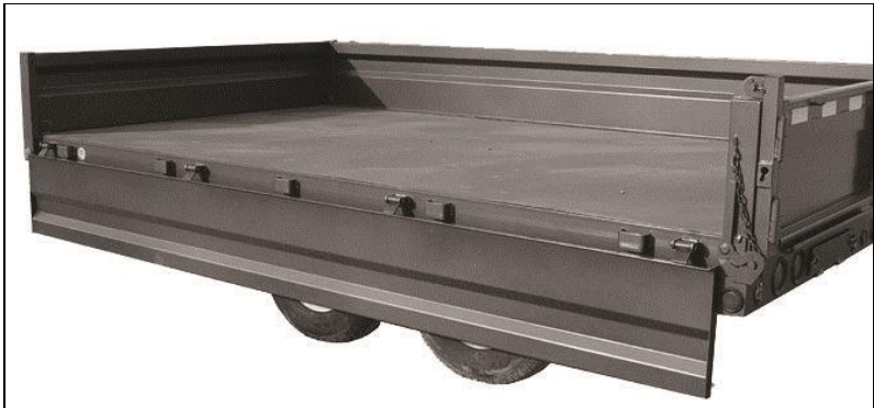
Left Side Panel Fully Lowered
