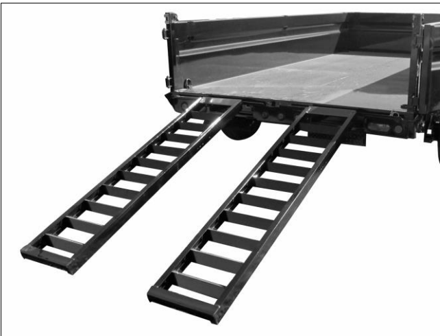
Dump Ramps Installed
