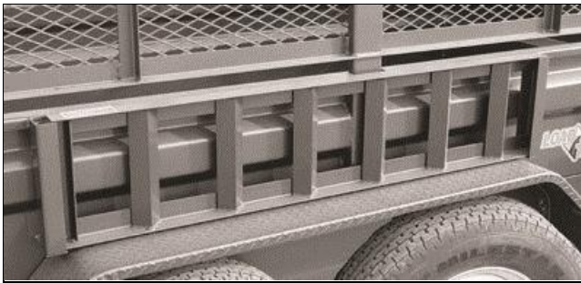
Over Fender Ramp Storage
