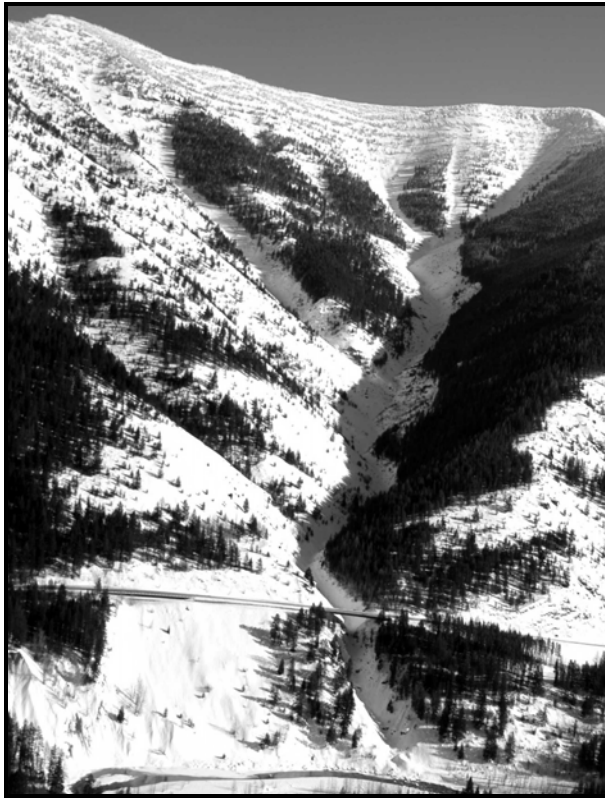
Figure 7: Aerial photo of west-facing Goat Lick Avalanche path showing multiple start zones and deeply channelized track under rebuilt highway bridge. Photo by D. Stoneman.
